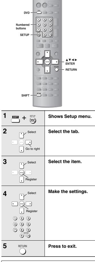
The settings remain intact even if you switch the unit to standby.
